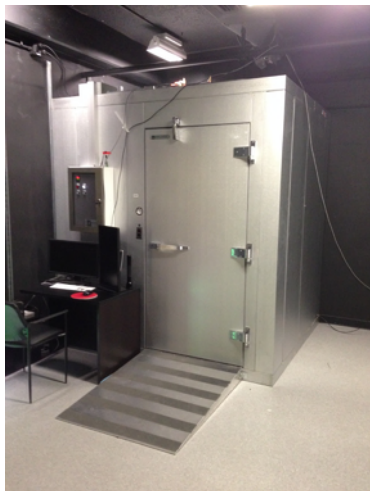
Figure S1. A view of the environmental chamber. Equipment is fully housed in the 37°C environmental chamber in order to avoid temperature fluctuations.
